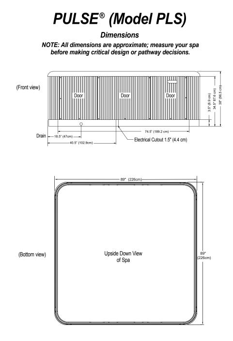
**NOTE:** Watkins Manufacturing Corporation recommends that the Pulse be installed on a minimum 4" (10 cm) thick reinforced concrete pad or structurally sound deck able to support the "dead weight" found in the spa specification chart.
