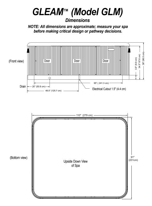
**NOTE:** Watkins Manufacturing Corporation recommends that the Gleam be installed on a minimum 4" (10 cm) thick reinforced concrete pad or structurally sound deck able to support the "dead weight" found in the spa specification chart.
