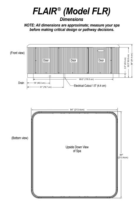
**NOTE:** Watkins Manufacturing Corporation recommends that the Flair be installed on a minimum 4" (10 cm) thick reinforced concrete pad or structurally sound deck able to support the "dead weight" found in the spa specification chart.
