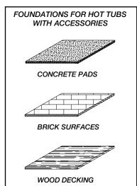
**NOTE:** In order for the spa to operate properly and the internal plumbing to drain completely, you must ensure that the spa is leveled after it has been installed.
