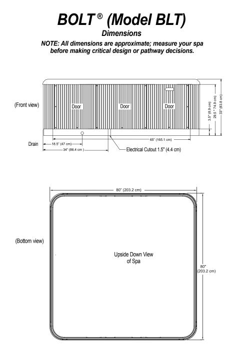
**NOTE:** Watkins Manufacturing Corporation recommends that the Bolt be installed on a minimum 4" (10 cm) thick reinforced concrete pad or structurally sound deck able to support the "dead weight" found in the spa specification chart.
