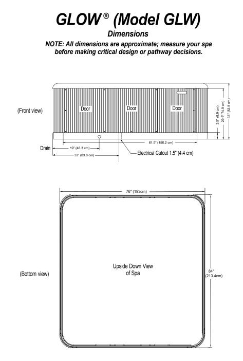
**NOTE:** Watkins Manufacturing Corporation recommends that the Glow be installed on a minimum 4" (10 cm) thick reinforced concrete pad or structurally sound deck able to support the "dead weight" found in the spa specification chart.
