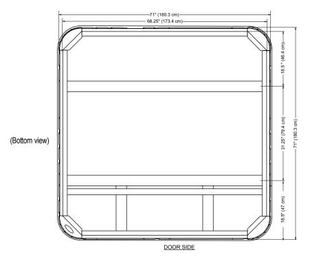
**NOTE:** Watkins Manufacturing Corporation recommends that the SX be installed on a minimum 4" (10.2cm) thick reinforced concrete pad or structurally sound deck able to support the "dead weight" found in the spa specification chart.
